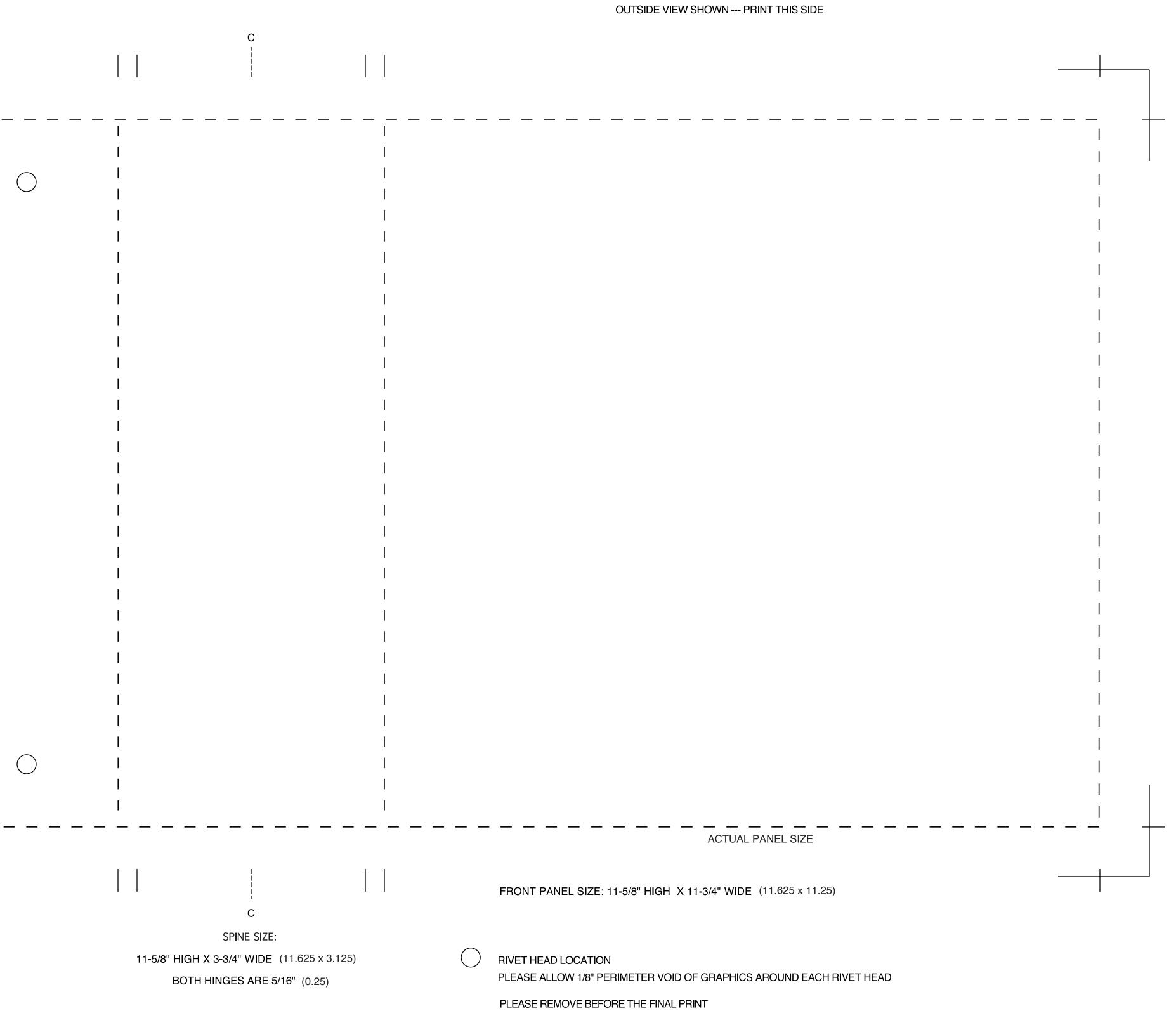
**3-PANEL WIDE SPINE** 11" X 8-1/2" SHEET SIZE PLUS 1/2" TAB ALLOWANCE 2.5" CAPACITY STRAIGHT D RING METAL LINER MATERIAL TEMPLATE 2.5" Cap-118.5-SD-FS-L
