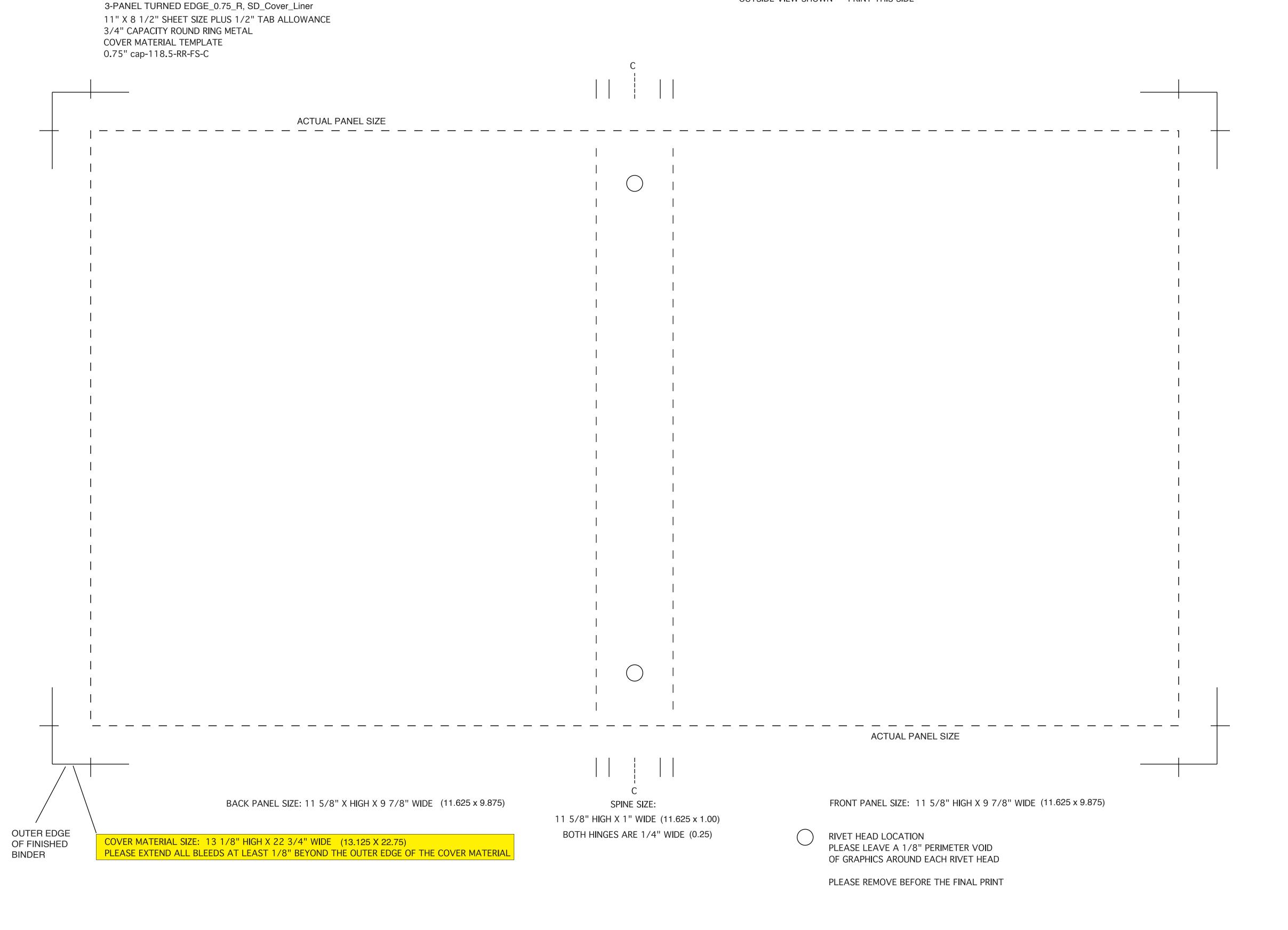
3-PANEL TURNED EDGE\_0.75\_R, SD 11" X 8 1/2" SHEET SIZE PLUS 1/2" TAB ALLOWANCE 3/4" CAPACITY ROUND RING METAL LINER MATERIAL TEMPLATE 0.75" cap-118.5-RR-FS-L
